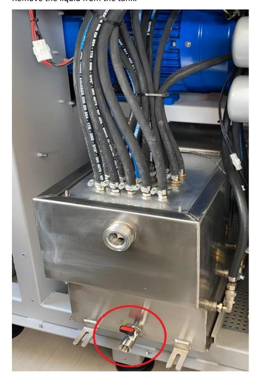
Step 3: Disconnect all Hoses and connectors the right and upside and remove the old tank.
