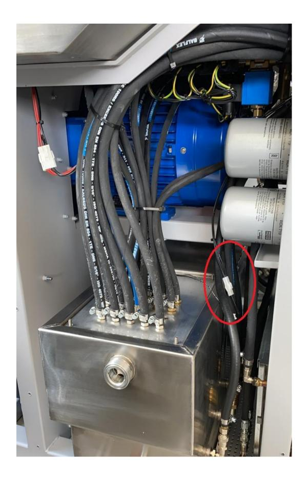
Connect the new heater tank and all the hoses to the new tank properly.
