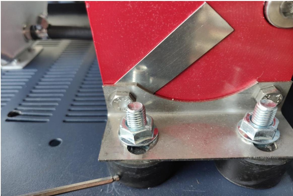
STEP.5 Make two holes to install the measure sensor.
