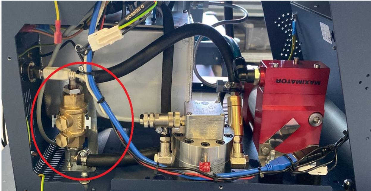
STEP.7 Connect the hose D port to the IN valve.
