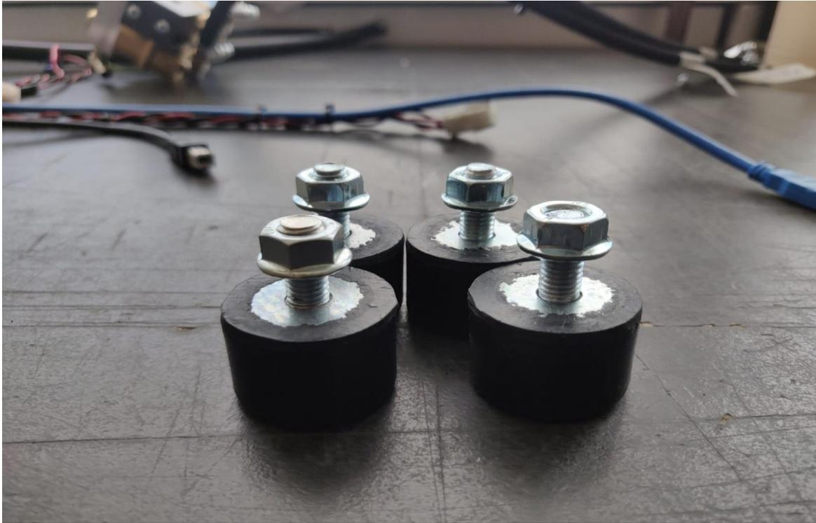
**Connect the new stands to down of the pump**
