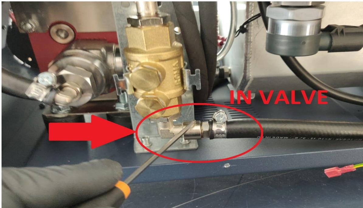
STEP.8 Connect the hose from the OUT valve to IN sensor measure.
