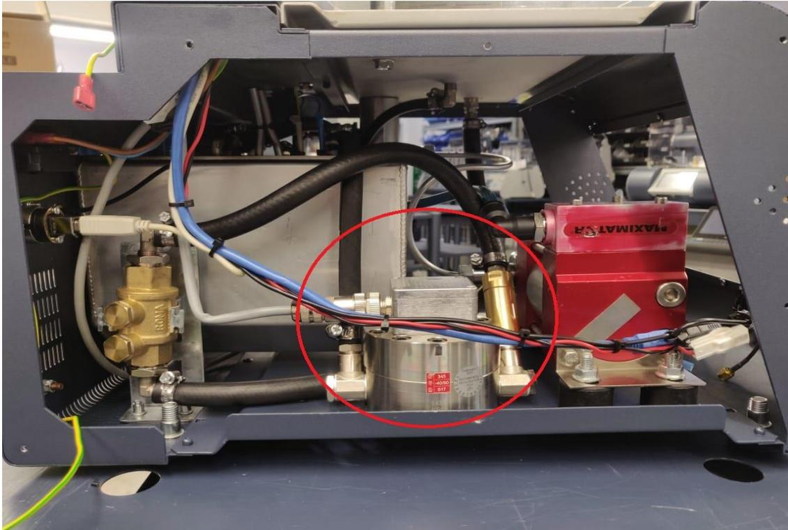
STEP.6 Make two holes to install the valve.
