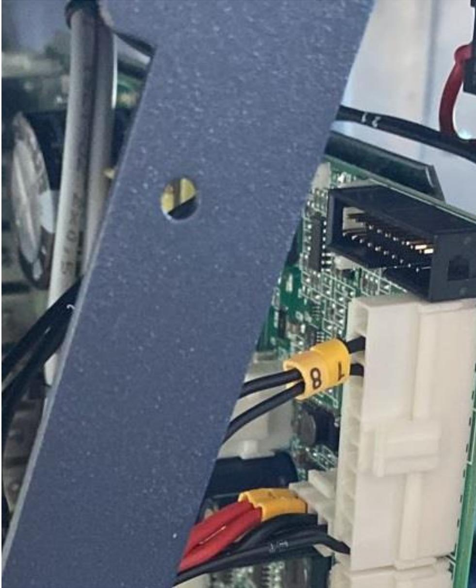
E. Connect the white connector from sensor measure.
