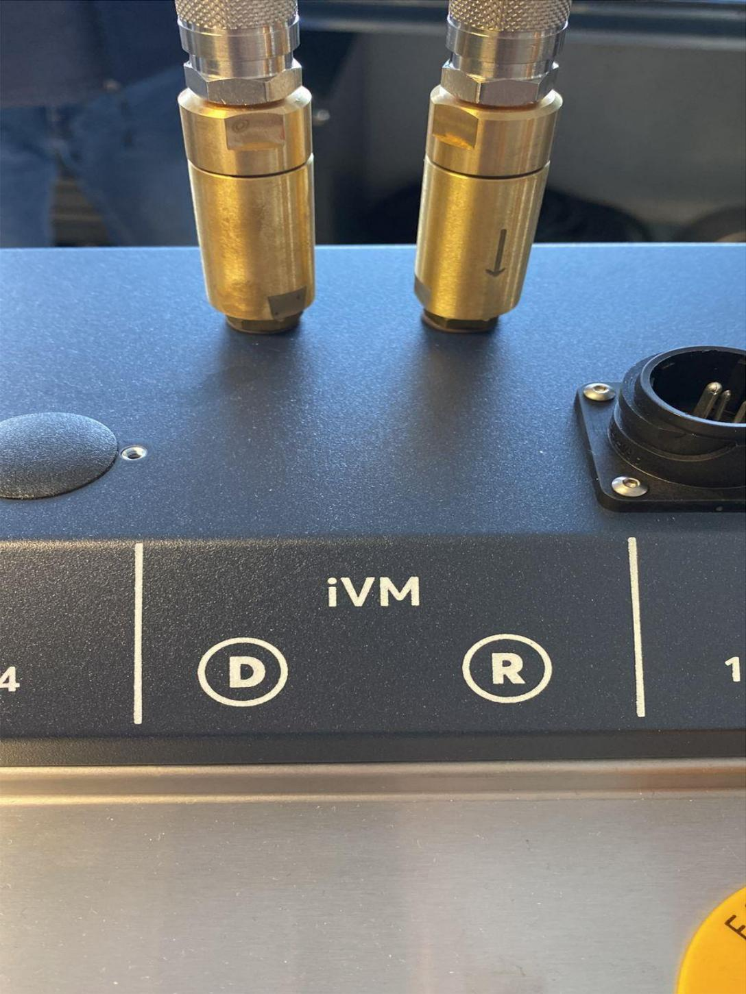
**Step 7: Place the new valves. Tighten the valve output hoses.**
