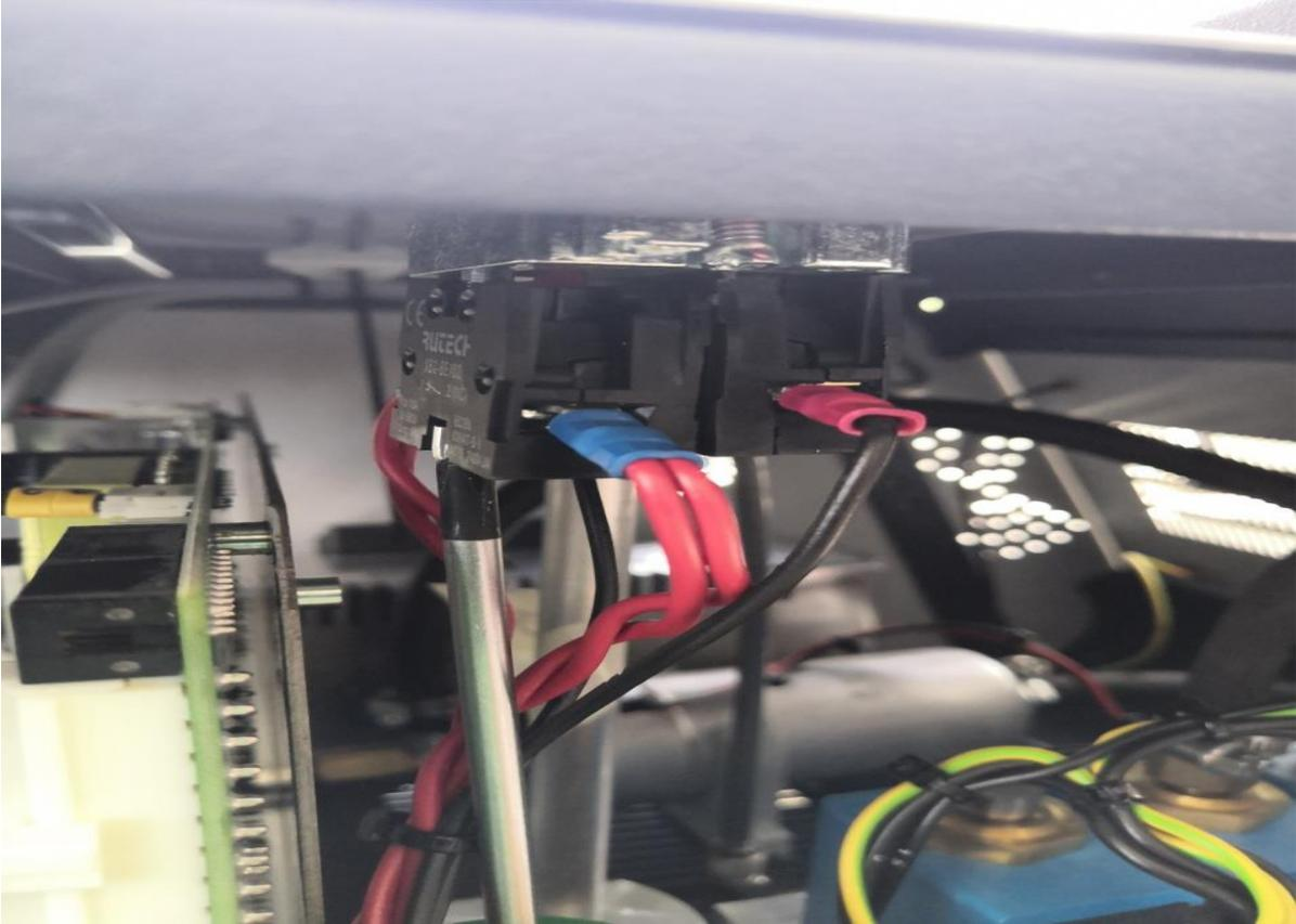
Step 12: Plug the cable adapter to the K20 connector on the PCB Board:
