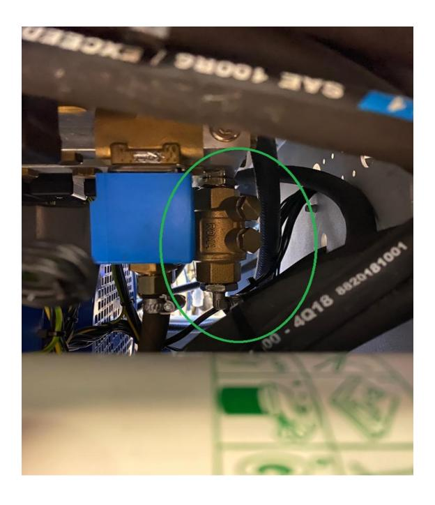
IMPORTNT check the arrow on the valve and connect to correct position.
