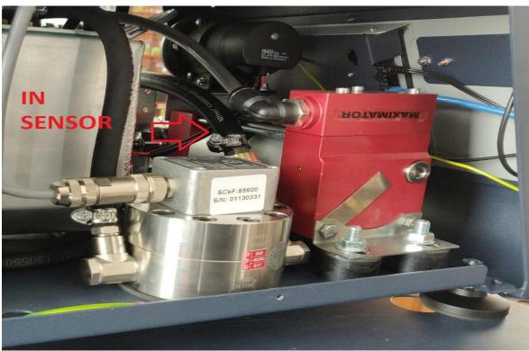
STEP.11 Connect the hose OUT Block electro valve to IN valve.
