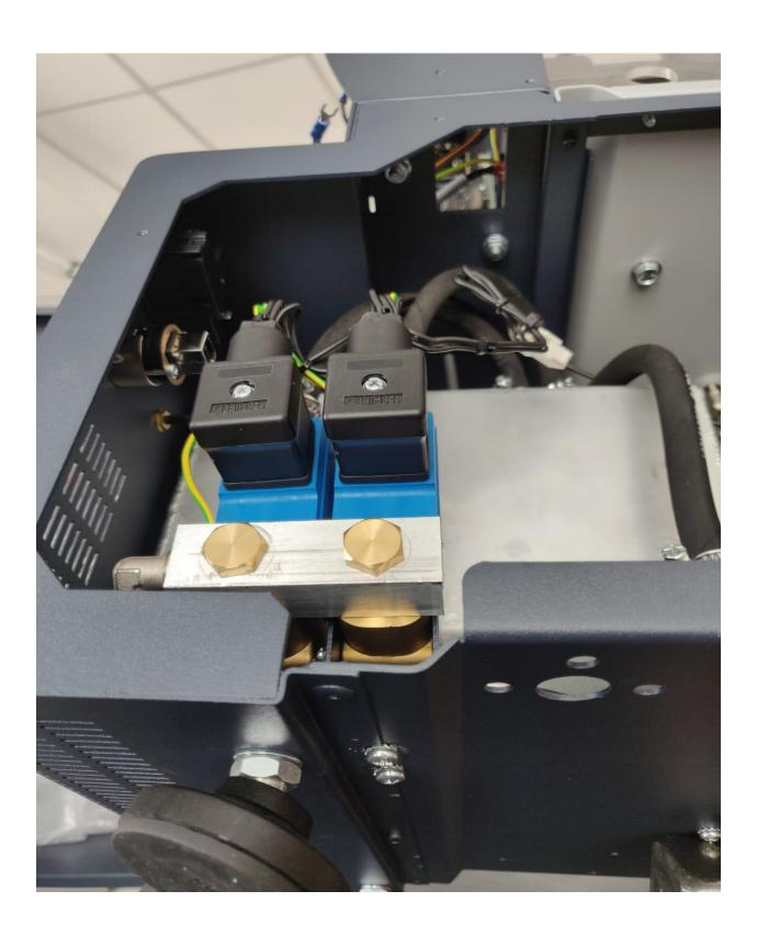
STEP.6 Make two holes to install the valve.
