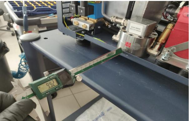
STEP.8 Check the position Sensor Measure and tired with 10Nm.
