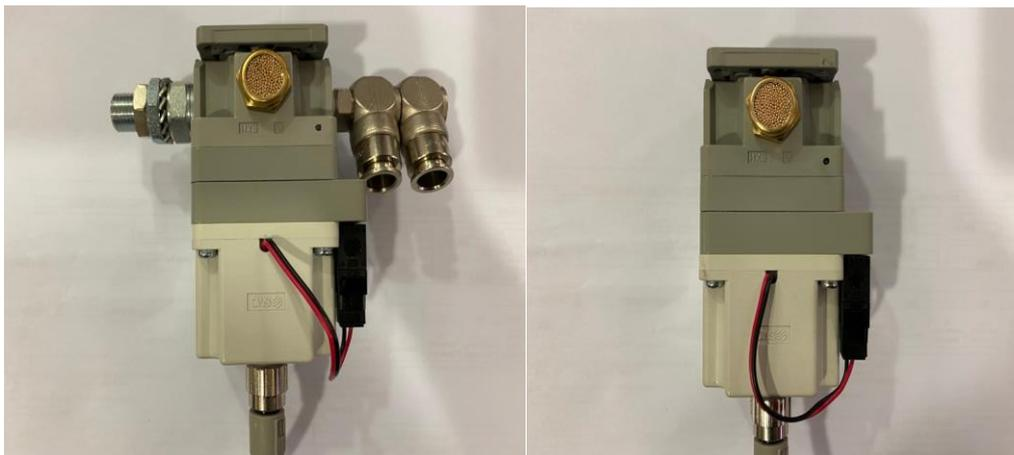
STEP.5.2a Connect the new parts to electronic SMC pressure air regulator.
