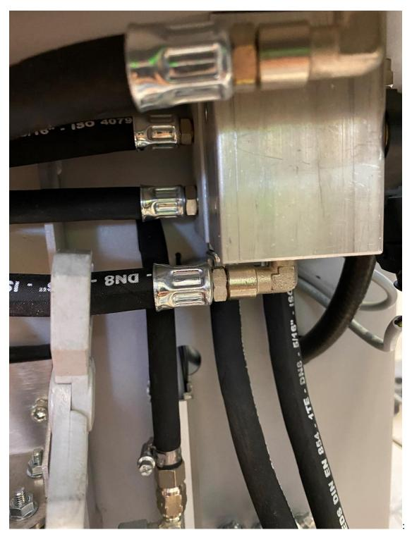
$\begin{array}{l} \text{Step 5} \\ \text{And connect the Valve important check the arrow on the valve} \end{array}$
