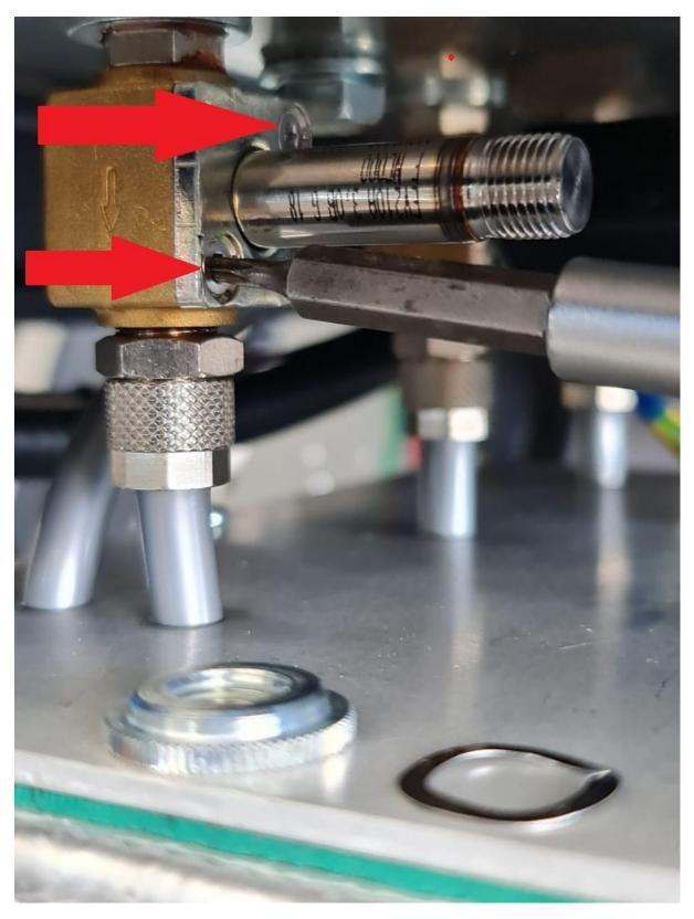
$\label{eq:Step 6} \mbox{Remove carefully the body and the pilot inside the valve.}$
