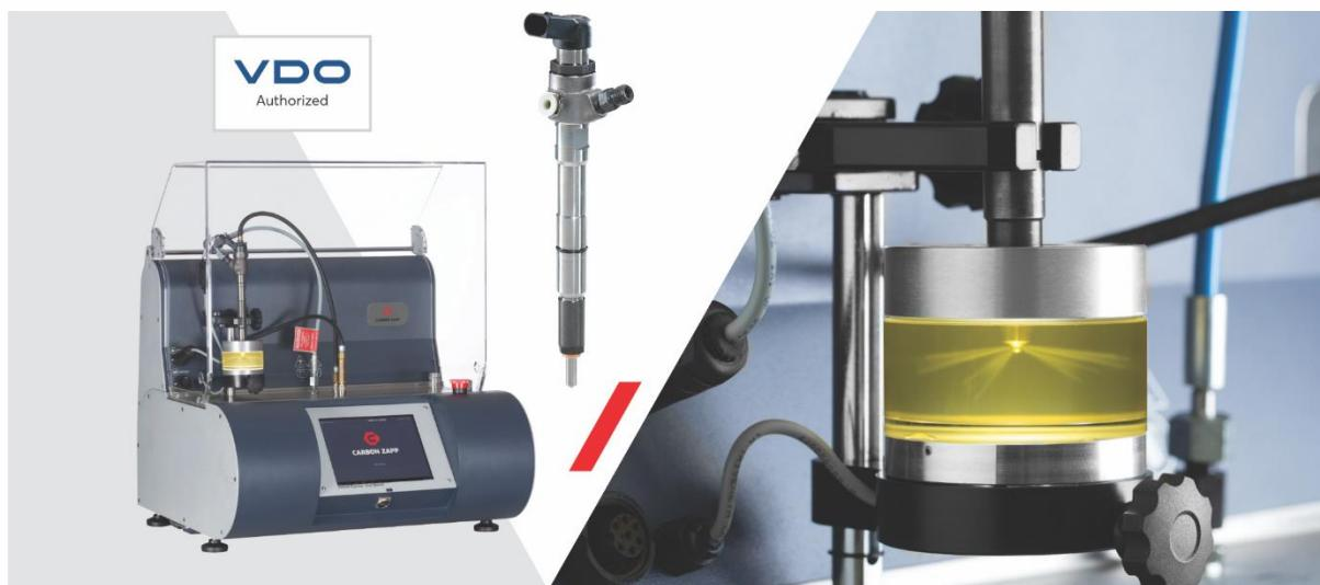
Carbon Zapp has optimized the testing applications of its diesel test benches allowing now the Authorized VDO DRS Partners equipped with Carbon Zapp CRU.2R units to also test, repair and code EU5 Common-Rail injectors by the Continental brand VDO thanks to the advanced testing capabilities of the bench to control the injectors implementing Energy Controlled signal.
