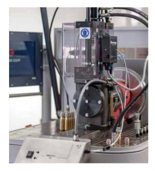
The **HK-1400A** has been engineered to be accurate and repeatable in testing Unit Injection Systems, yet is affordable for all Diesel workshops worldwide.
